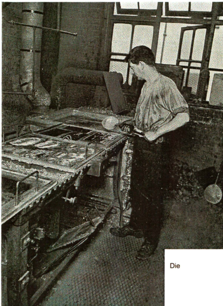
Above: backing the thin copper shell with molten type-metal; Right: stages in making the master plate
