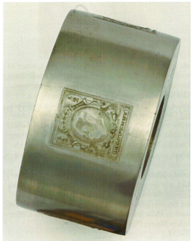
Right: transfer roller to make dies for striking leads.
