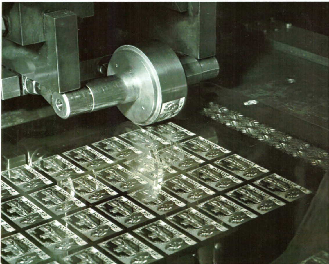
Below: transfer roller rocking the image of the Castles 2/6d to create the recess plate
